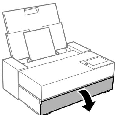
7. Slide out the output tray to its maximum position.
