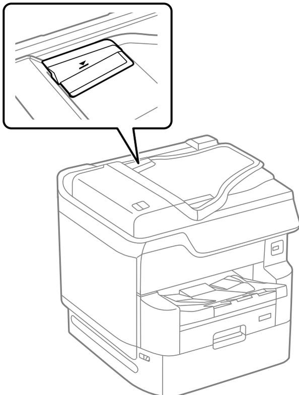
■ **The original slips when paper dust adheres to the roller.**
