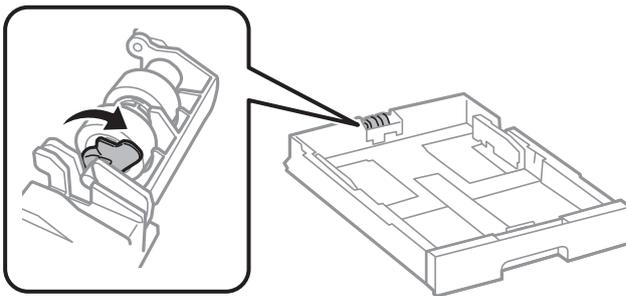
11. Slide the maintenance roller toward the lever, and then remove them by taking the shaft out of the holder.
