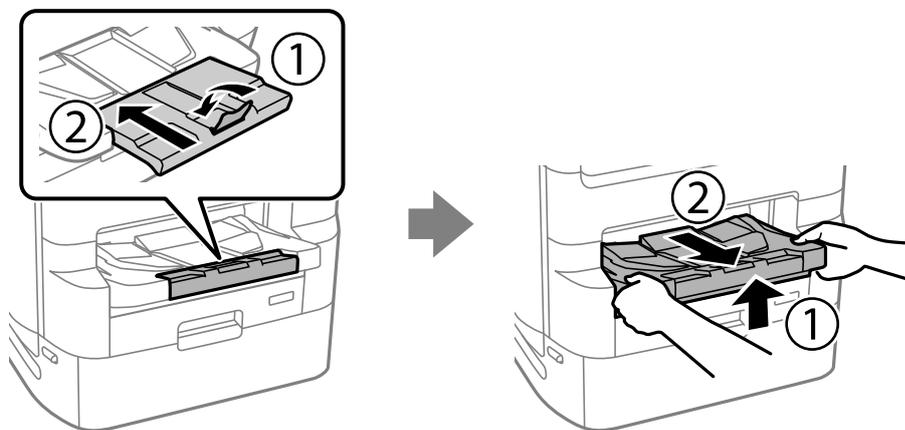
4. Remove the paper cassette unit from its box, and then remove any protective materials.
