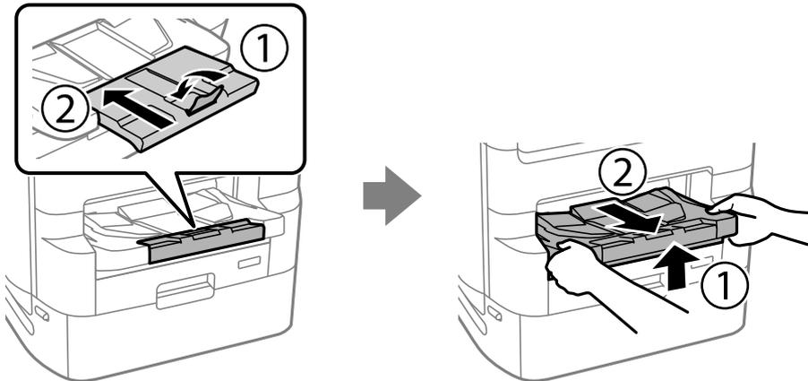
4. Remove the printer stand from the box, and then remove any protective materials.
