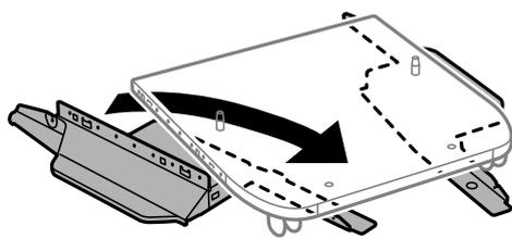
7. Secure the stands with the attachments and screws.
