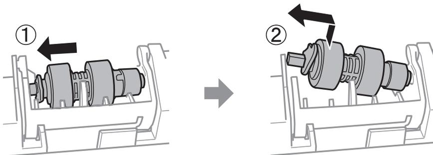
12. Insert the shaft of the new maintenance roller into the hole in the holder, and then slide the shaft on the lever side along the slot while it is facing the flat surface at the front.
