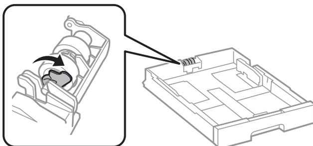
13. Slide the maintenance roller toward the lever, and then remove them by taking the shaft out of the holder.
