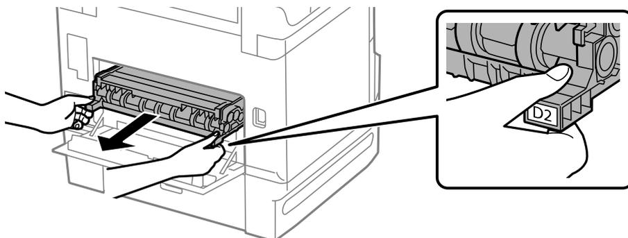
6. Remove the cover inside the back of the printer.
