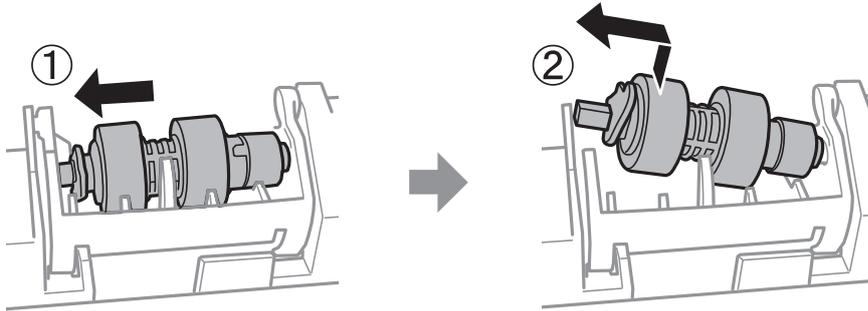
14. Insert the shaft of the new maintenance roller into the hole in the holder, and then slide the shaft on the lever side along the slot while it is facing the flat surface at the front.
