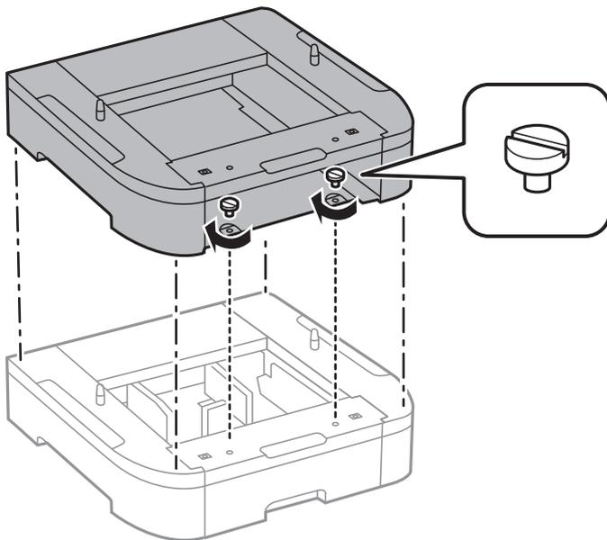
9. Lower the printer gently onto the paper cassette unit aligning the corners, and then secure them with the screws.
