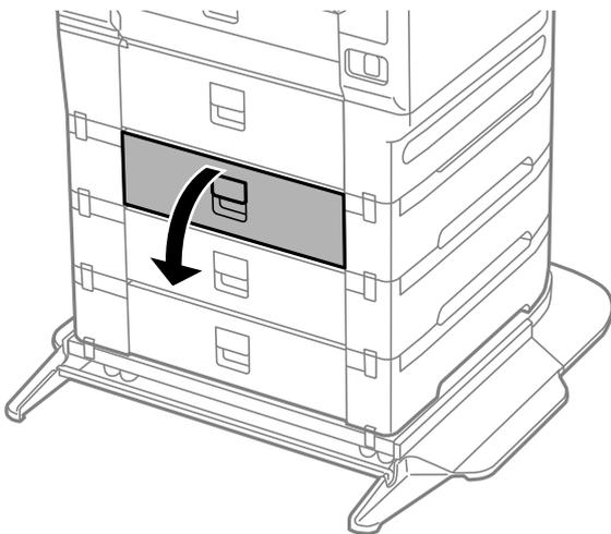
5. Remove the screws by a screwdriver and remove the cover on the rear of inside the printer.
