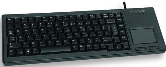
Slim, compact keyboard with integrated Touchpad. Gold Crosspoint keyswitches ensure operational reliability and durability. For industrial applications, in IT, Point of Sale and medical facilities. Easy installation and fixation in kiosks and keyboard drawers.
