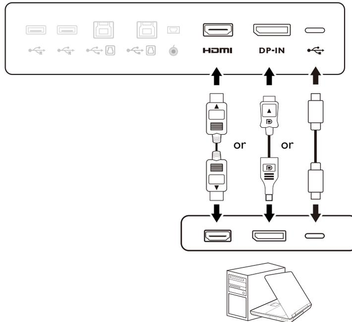
2. Connect the other end of the video cable to an appropriate port of a digital output source (e.g., a computer).
