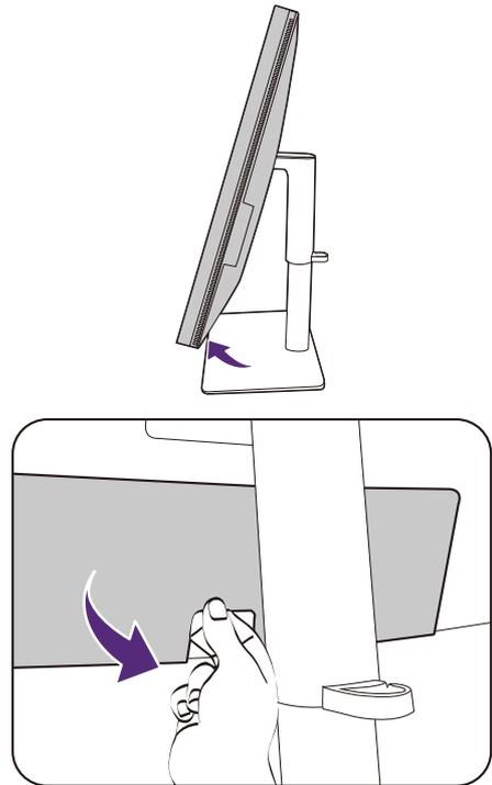
Protect the monitor and screen by clearing a flat open area on your desk and placing a soft item like a towel on the desk for padding, before laying the screen face down on a flat clean padded surface.
