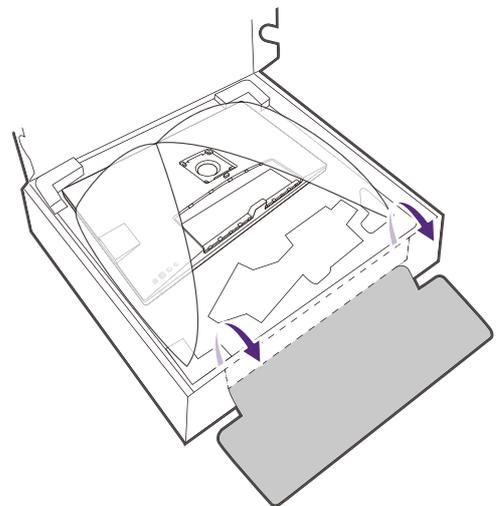
Orient and align the stand arm with the monitor, then push them together until they click and lock into place.
