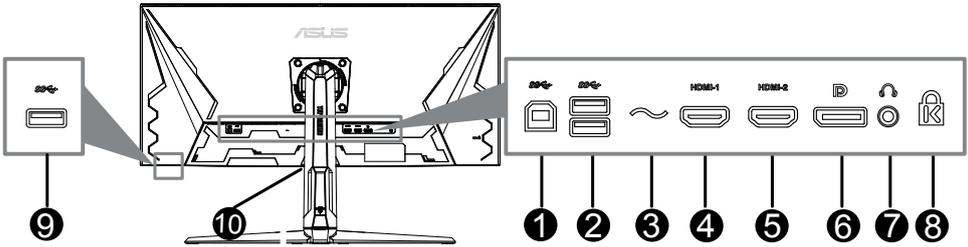
**9** This port is for connection with a USB upstream cable. The connection enables the USB ports on the monitor.
