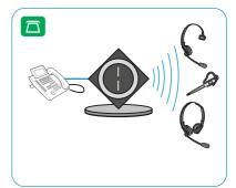
Place the base station at a minimum distance of 15 cm from the fixed line phone.
