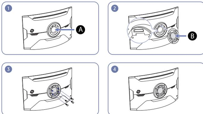
**A** Attach the BRACKET WALL here
