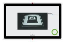
If the screen image is not in the center, the calibration will fail. Please make sure the PointWrite module is attached to the projector properly.
