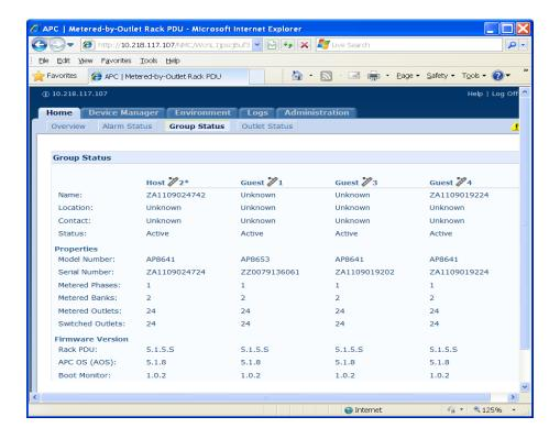
Most of the web pages under the Home, Device Manager, and Environment tabs allow you to switch between Rack PDUs for viewing status and configuration/control. This switching is accomplished by selecting the Rack PDU Display ID of the unit you would like to view. This is located at the top right of each table that supports multiple Rack PDUs. The Host Rack PDU that you are logged into is always denoted with an asterisk (\*) following the Display ID.
