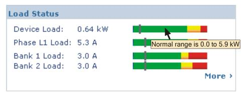
Click **More** to go to the **Device Manager** tab to configure thresholds and to view and manage peak load information.
