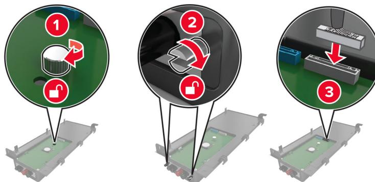
6 Open, and then remove the controller board access cover.
