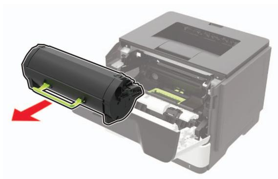
3 Remove the used imaging unit.
