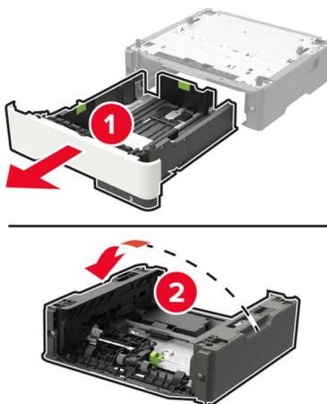
**5** Remove the used pick roller assembly.
