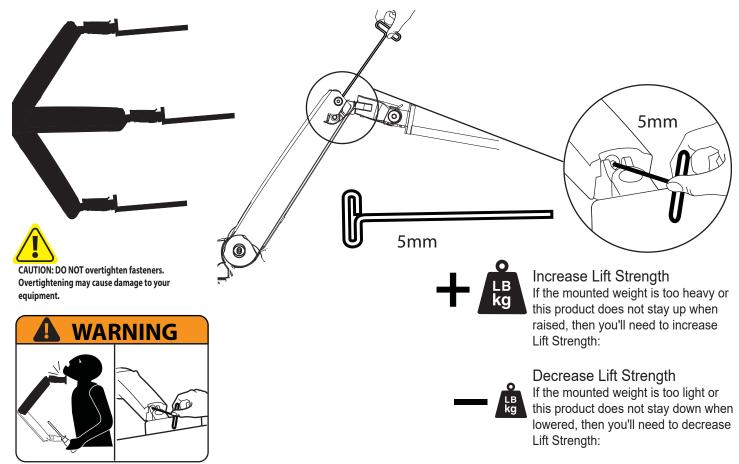
WARNING! Stored Energy Hazard: The arm mechanism is under tension and will move up rapidly, on its own, as soon as attached equipment is removed. For this reason, DO NOT remove equipment unless the arm has been moved to the highest position! Failure to follow this instruction may result in serious personal injury and/or equipment damage!
