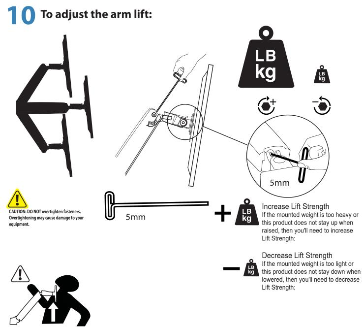
WARNING! Stored Energy Hazard: The Riser mechanism is under tension and will move up rapidly, on its own, as soon as attached equipment is removed. For this reason, DO NOT remove equipment unless the Riser has been moved to the highest position! Failure to follow this instruction may result in serious personal injury and/or equipment damage!
