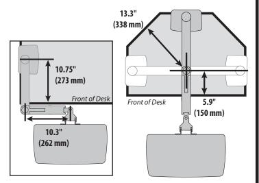
Grommet hole can be located anywhere along this arch.
