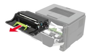
**Warning—Potential Damage:** Do not expose the imaging unit to direct light for more than 10 minutes. Extended exposure to light may cause print quality problems.
