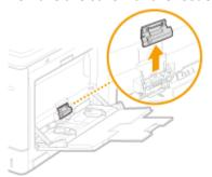
4 Pull out the upper feeder roller.
