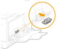
5 Wipe off the glue residue sticking to the feeder roller.
