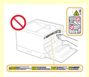
Do not carry the machine with the optional paper feeder or cassette feeding unit installed. Otherwise, they may fall, resulting in injury.
