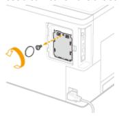
2 Open the ROM cover, and remove it in the direction indicated by the arrow.
