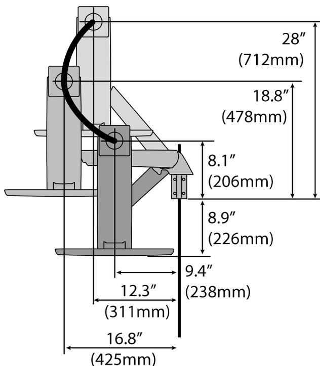
Top view showing range of motion when pulled out from the wall.
