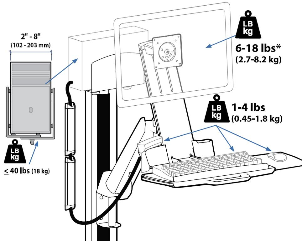
\*The Combo Arm can be modified to mount displays up to 25 lbs (11.3 kg), however display lift and tilt motion will not be possible if this option is chosen. Refer to special instructions on page 14.
