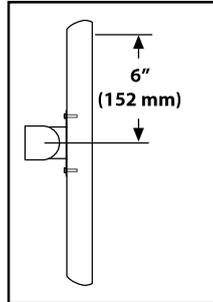
Mounting height assumes there is a 6" (152 mm) distance between the center of your monitor mounting holes and the top of the screen. If your distance is smaller, you should increase mounting height accordingly, if your distance is larger, you should decrease your mounting height accordingly.
